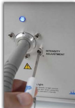
Intensity adjustment, with knob removed, performed with adjustment tool
