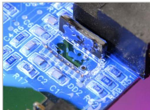
Cured Dual-Cure Coating Under PCB Component
